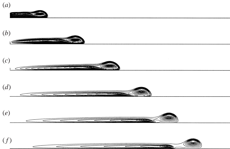
FIGURE 11. The vorticity field for the parabolic discharge velocity ( T^* = 6 and Re = 2500 ). The formation times are (a) t^* = 4.3 , (b) t^* = 7.2 , (c) t^* = 9.6 , (d) t^* = 14.4 , (e) t^* = 19.2 and (f) t^* = 24.0 . The non-dimensional vorticity contour lines are plotted for the range of \omega = 0.17 to 17 with an increment of 0.83.
